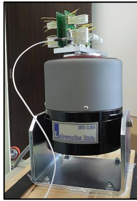
Figure 9 PCB with mated FFC and connectors were placed in position X and Y with electrical connected on the electrodynamic shaker for one month.
