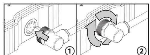
① Ensure the circular multipole plug align with the receptacle on the sensor module by following the locking guide.
