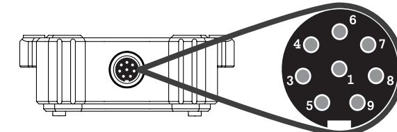
Sensor DB-9 Male cable connector pin-out
