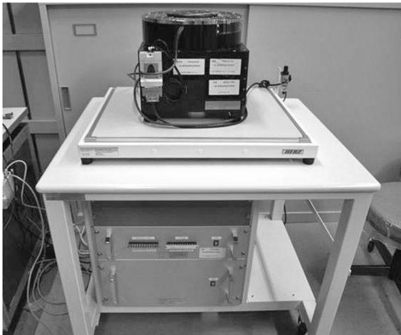
SelfA47 Precision Rotary Table System for Angular Standard (Japan) - Source: National Metrology Institute of Japan (NMIJ)
